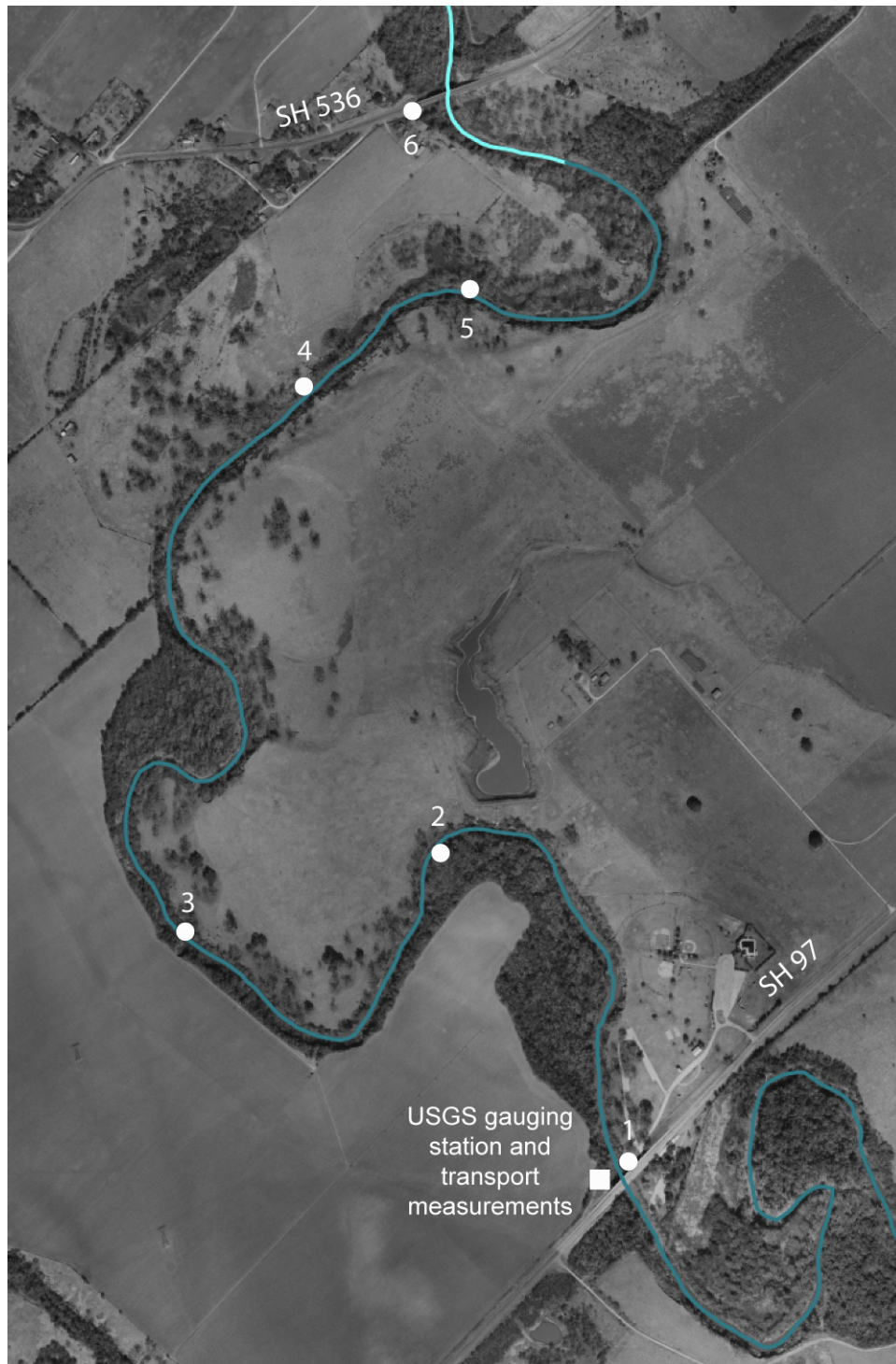
Figure 1. The Floresville reach. Locations of channel cross-sectional survey and boundary material sampling shown by circles. Location of USGS streamflow gauging and sediment transport measurements shown by square.
